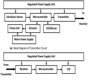
(b) Block Diagram of Receiver Circuit
