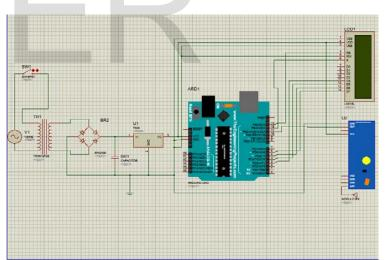
Fig. 8. Circuit Diagram of Receiver System on Proteus 8.1
